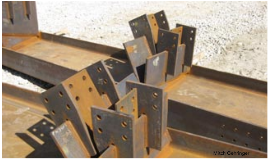
Many of the connections required multiple connection plates at various angles, posing challenges to both the detailer and the fabricator.
